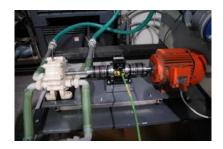
Fig. 10: Torque transducers conected between turbine and motor
