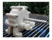
Fig. 8: Model of side-channel turbine
