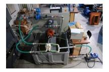
Fig. 11: Measurement circuit for turbine with divided suction
