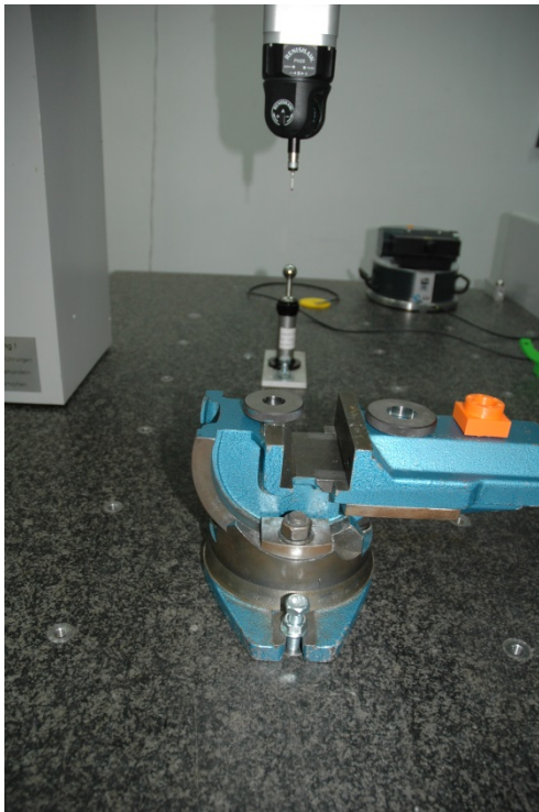
Figure 2: Measuring station, PH20 probe head and standard ring
