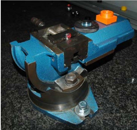
Figure 3: The holder used in 0,5 inch SMR measurements
