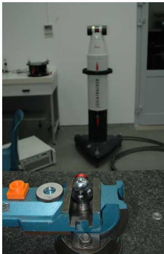
Figure 2: Measurement station with the 1,5 inch SMR holder
