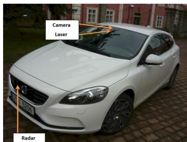
Figure 1: Position of camera, radar and laser
